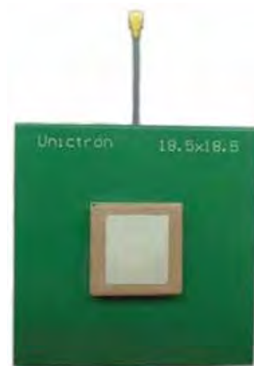
SMD patch antenna 18 × 18 mm on the demo board.
